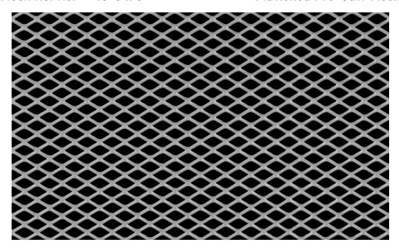
LW Aperture:6.00mmStrand Width:1.30mmSW Aperture:3.45mmThickness:0.70mmWeight:2.35 kg / m2Open Area:57%
